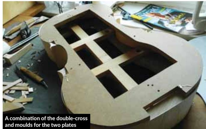
A combination of the double-cross and moulds for the two plates
