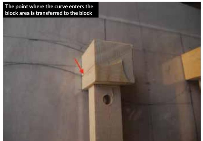
The point where the curve enters the block area is transferred to the block
