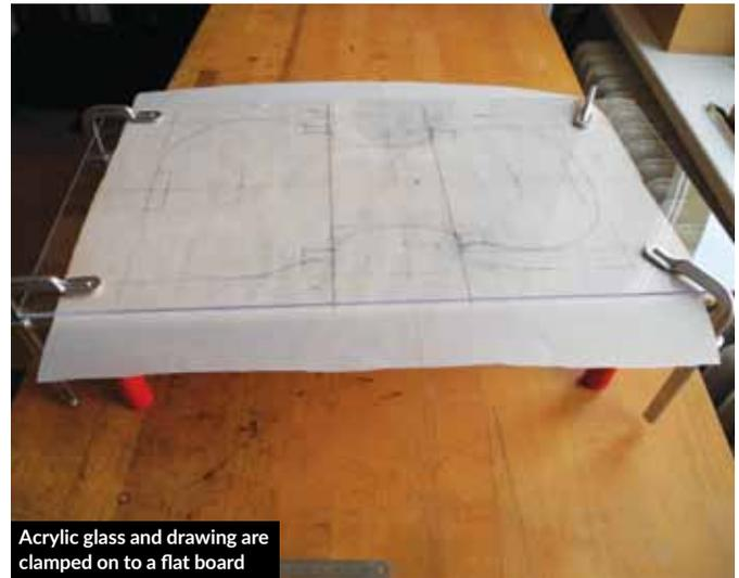
Acrylic glass and drawing are clamped on to a flat board
