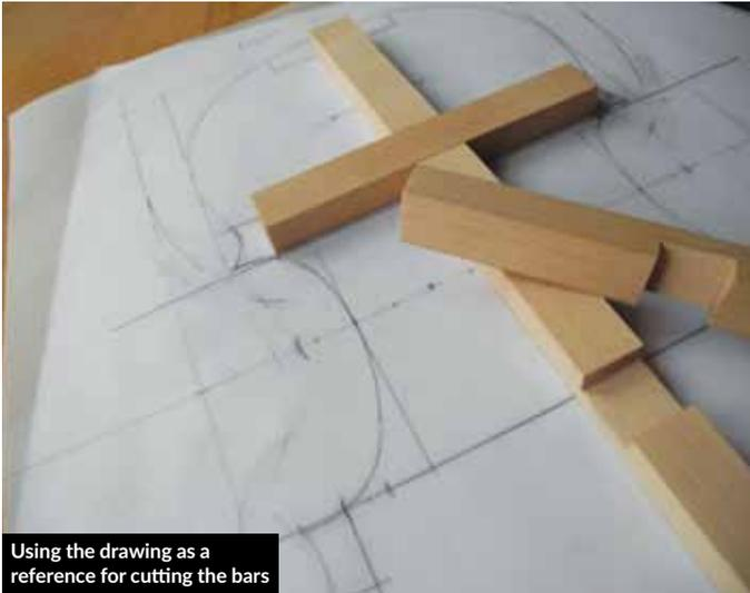
Using the drawing as a reference for cutting the bars
