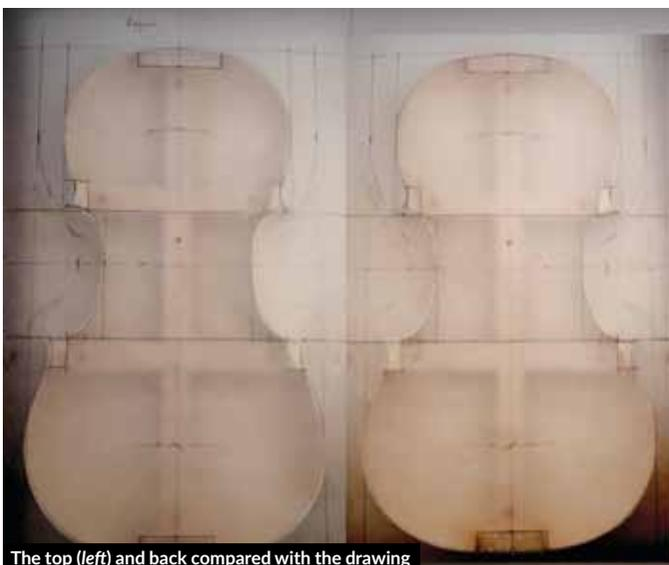
The top (left) and back compared with the drawing
