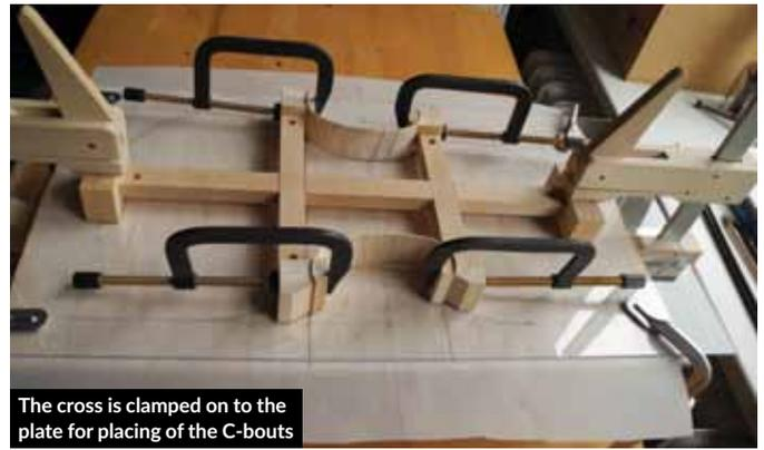
The cross is clamped on to the plate for placing of the C-bouts
